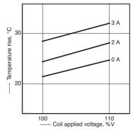
4-(2) Influence of adjacent mounting Tested sample: DS2Y-S-DC12V, 10 pcs. Ambient temperature: 20°C 68°F
