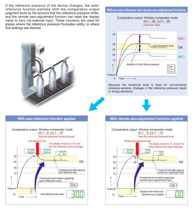
When auto-reference input is applied, the reference pressure "30" is added to the threshold level. If the reference pressure changes to "20" or "40", the auto-reference input compensates for this every time by changing the threshold level, so any variation in the filling pressure can be ignored.
