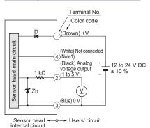
Notes: 1) In case the sensor head is used independently, insulate the white lead wire (terminal No.4) and keep it open.
