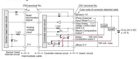
Notes: 1) Select and use the auto-reference function and remote zero-adjustment function. 2) Set the output load resistance during analog current output to 250  $\Omega$  (max.) 3) Note that a voltage of +5 V or higher is generated during analog current output.
