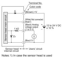
independently, insulate the white lead wire (terminal No.4) and keep it open.
