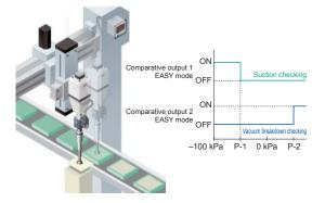
Reference pressure alarm output is possible during reference pressure checking!
