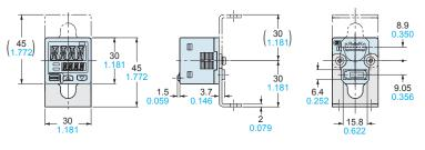
Material : Cold rolled carbon steel (SPCC) (Uni-chrome plated) Two M3 (length 6 mm 0.236 in) screws with washers are attached.
