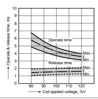
4.-(2) Operate & release time (180 mW) Tested sample: PA1a-24V, 20 pcs.
